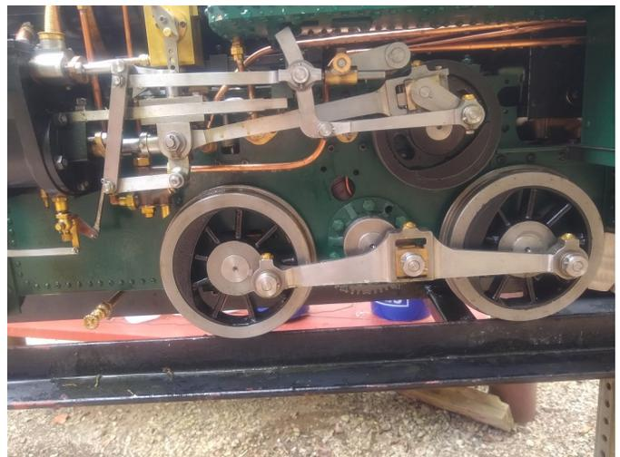
Rick's Engine's Intricate Valve Gear
