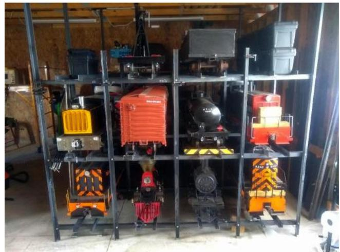
Once we were satisfied that the rack was not going to move, we started loading some of our equipment from individual stands using our train elevator. Since the top level is 2-1/4" higher than our elevator can reach, we created a short wooden ramp to compensate for the difference.
