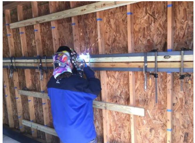
Once all the track subassemblies were welded, it was time to weld on the laterals to create the 3 level subassemblies. We again employed our wall-mounted jig, then clamped the laterals on the rail subassemblies and welded each
