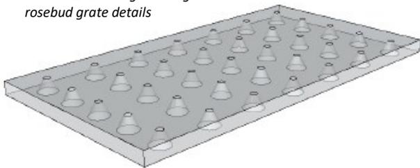
The drawing above shows how the holes are reamed out on the air in-take side and are narrowed for maximum velocity on the fire side of the grate.
