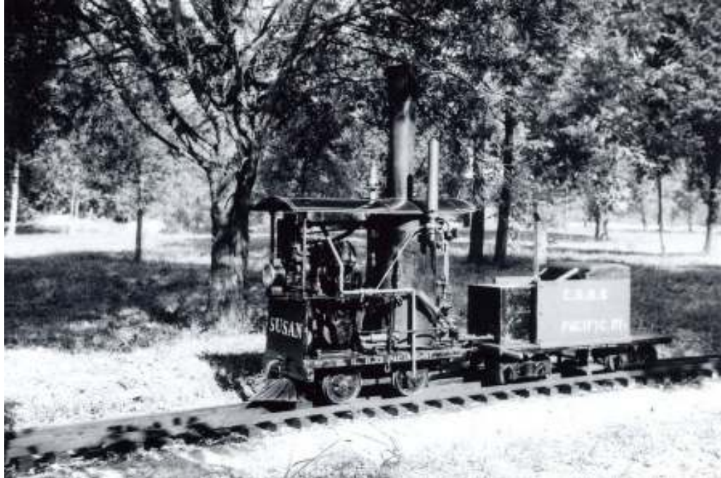
Here is proof that Susan once was a painted lady complete with stripes. The tender has the trucks with single springs and a hand brake against the track.
