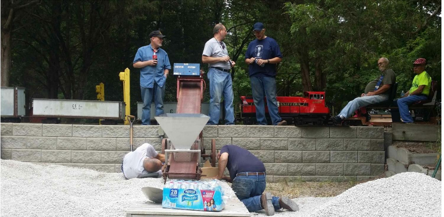
**Repairing Gravel Loader:** “The conveyor belt began to tear and ... uh-oh ... there was a wasp’s nest under there.” Fortunately, the belt was “wired” back together and gravel loading continued. Left to right: Chuck Balmer, Denis Larrick, Don Frozina, Roger Heurich, Tom Tekulve. Working on the loader: Ed Habel and Carl Schwab. Others not shown: Dave Sams, Ray McNeil, Bill Mense, Jim Balmer & Harvey Bond.
