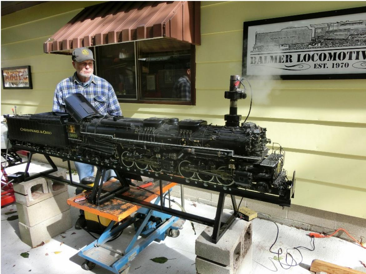
We got the Allegheny out and test fired it on our rolling stand and ran the engines on steam for the first time. The engines ran very well once we got them rolling and would stop and restart after that with no issue. We had a few of the accessories that worked like the air powered drain cocks and steam turbo generator.
