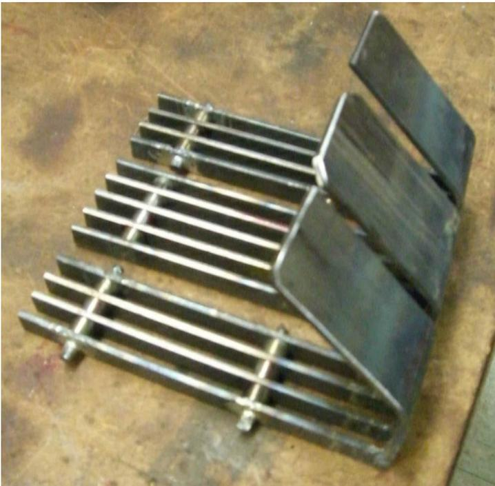
The grates with integral arches, split into 3 parts to fit through the fire door. The grates can be inserted by angling the arch into the roof of the fire box and sliding it down through the door. Insert the side grates first then the center one.
