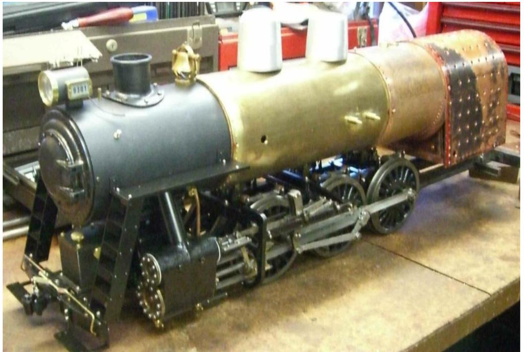
I also discovered that the piston valves were so tight that I had to use a wooden dowel and a hammer to drive them out of the valve port spools. I used an expandable reamer to open the port spools so that the valves would move freely. The entire chassis was cleaned and repainted before being reassembled. Much of the valve gear was made from brass or bronze castings and coated with lead or tin solder to make them look like steel. Much of this coating had to be removed.
