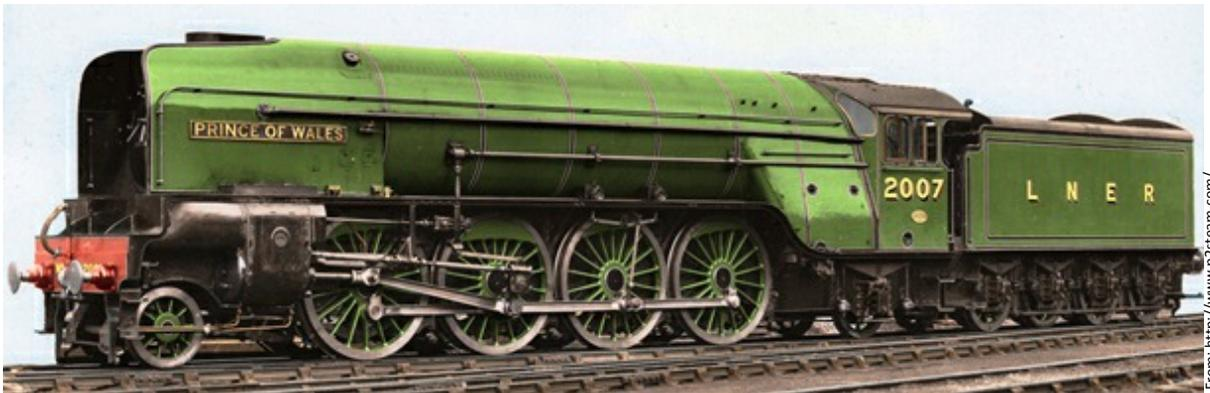
Whereas, between 1905 and 1930 the 2-8-2 type was built in far larger numbers than any other type in the United States (around 14,000 total),\* the Mikado type was not common in Great Britain. Only six of the class were built and these in 1935-1936 to handle passenger trains over a "harsh" section of the London and North Eastern Railway. One of the six was the prototype for John Cottam's IMLEC winner.
